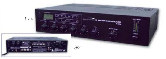
Our professional 30 Watt PA amplifier features a digital 30 station preset FM/AM tuner, built-in telephone paging, voice activated priority paging and music on hold circuits. Input connections include two locking Cannon type XLR connectors, one 1/4" microphone connector, one RCA aux input. Outputs include 4 ohm, 8 ohm, and 25/70 volt. It has a 30 Watt RMS at less than 1.0% distortion. It has a dual voltage 12OV/220V AC for 50/60 Hz. A rack mounting kit is included.
